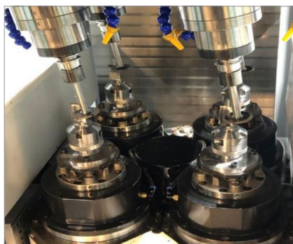
图10 4件叶片阵列抛光加工工况 Fig.10 Array polishing for 4 blades
